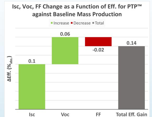
Breakdown of each component's effect on overall efficiency from the data shown in the table
