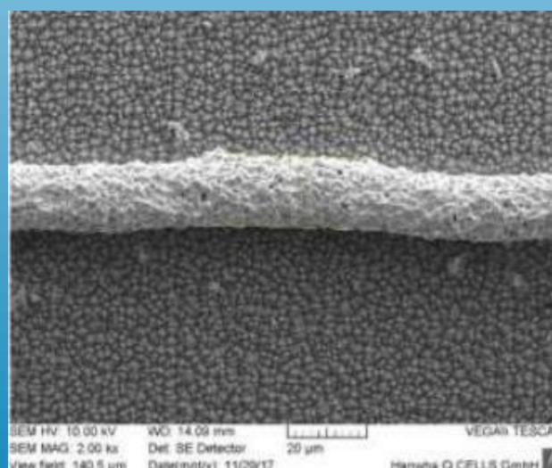
Finger line printed by PTP™ process using 20um tape - fired line widths are ≤20µm
