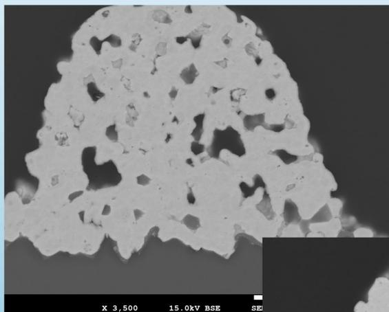
In order to maintain sufficient line conductivity with the reduced finger line volume, the time/temperature sintering characteristics of standard pastes need to be altered significantly
