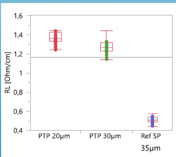
Line resistance at 20µm, 30µm tape widths versus a screen printed reference paste through a 35µm opening – the increase in line resistance is due to the decrease in paste volume
