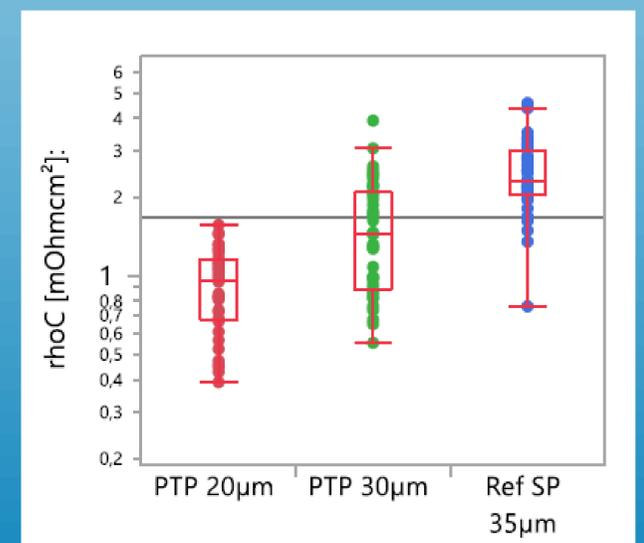
Contact resistivity of PTP™ versus a screen printed reference – after significant paste and glass modifications, we are able to achieve even lower rhoC values than that of the reference
