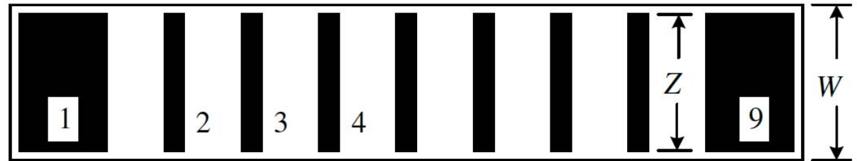
Linear equivalently spaced TLM (i.e., ladder)
